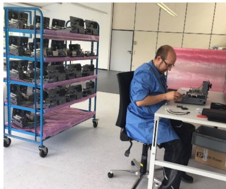
Assembly at ESD work places
